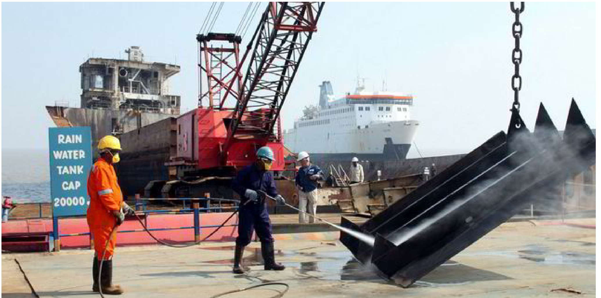
Steel plate removed from a ship being cleaned before further cutting, at Shree Ram recycling yard, Alang. Oily waste is channeled into a tank nearby Photo: TradeWinds
